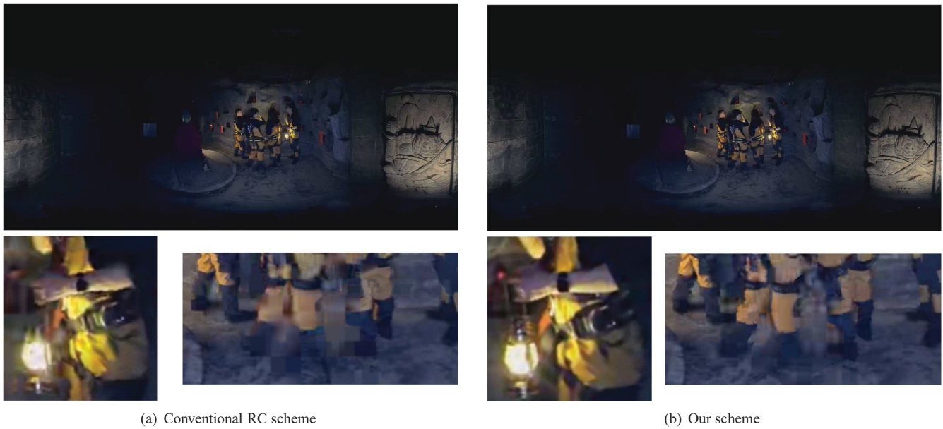
Fig. 6: Visual quality of Dianying compressed at 158 Kbps by HM-15.0 with our and conventional RC [14] schemes. Note that this figure shows the 68-th frame of compressed Dianying .
